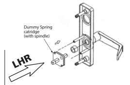
2. ROTATE LEVER TO DESIRED HAND, INSERT COLLAR, SPRING CATRIDGE IN ESCUTCHEON PLATE
