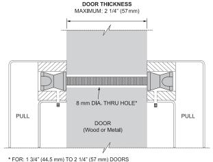
\* FOR: 1 3/4" (44.5 mm) TO 2 1/4" (57 mm) DOORS USE THE M6 X 72 mm THREADED BOLT
