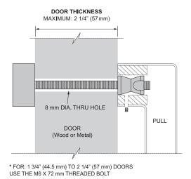
$^{\star}$  FOR: 1 3/8" (35 mm) TO 1 3/4" (44.5 mm) DOORS USE THE M6 X 60 mm THREADED BOLT
