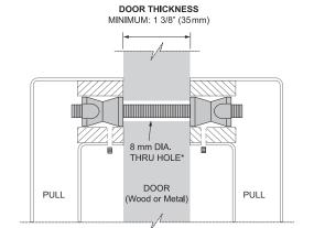
\* FOR: 1 3/8" (35 mm) TO 1 3/4" (44.5 mm) DOORS USE THE M6 X 60 mm THREADED BOLT
