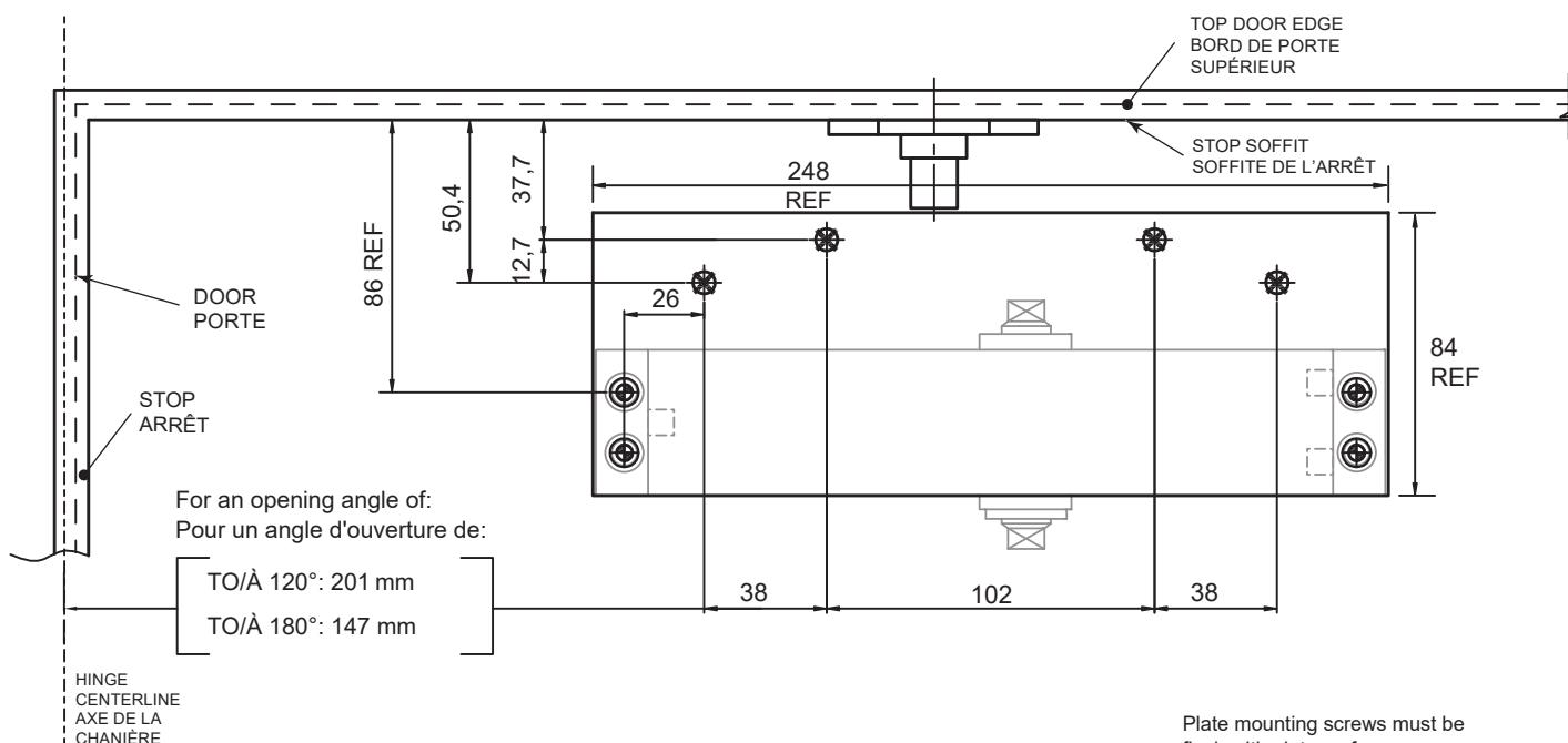
Plate mounting screws must be flush with plate surface.
